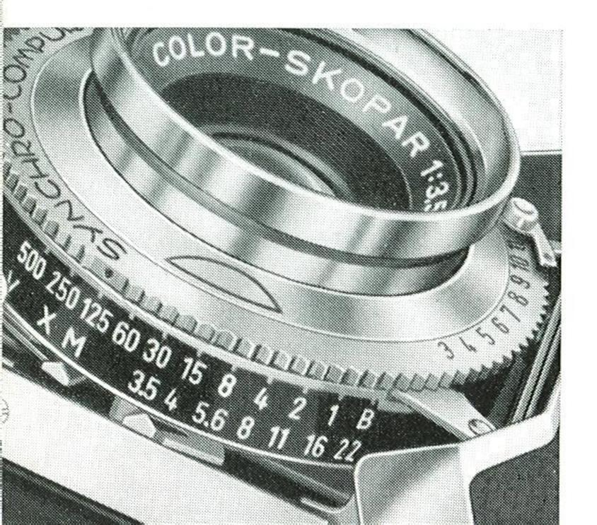
The aperture and speed settings are coupled. The combinations of apertures and shutter speeds are expressed in terms of "exposure values". The exposure value setting required depends on the prevailing lighting conditions, and once set, it gives the right aperturespeed combination for correct exposure. Every single exposure value thus corresponds to a whole range of equivalent aperture-speed combinations (e. g. 1/60 second at f/5.6, 1/30 second at f/8, 1/15 second at f/11, and so on).
